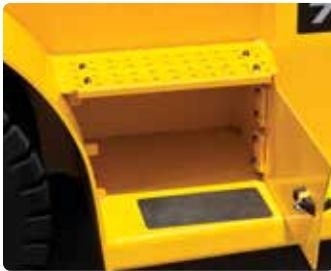
Large Tool Box Additional tool box located in machine side for operator's convenience.
