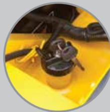
**Key-locking fuel cap with air vent**
