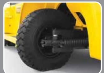
**Fully hydrostatic power steering**
