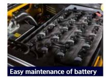
The battery cover opens fully with the assistance of a gas strut that locks when fully opened to give easy access to battery and prevent the hood from dropping. An automatic electrolyte liquid filling machine is offered as an option for hassle -free battery maintenance.
