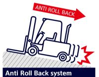
Anti roll-back system offers protection against the machine rolling back on a ramp in combination with exceptional ramp start capabilities.
